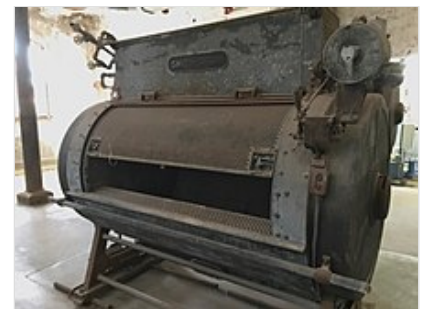
A Smith Drum laundry machine in the outbuilding
